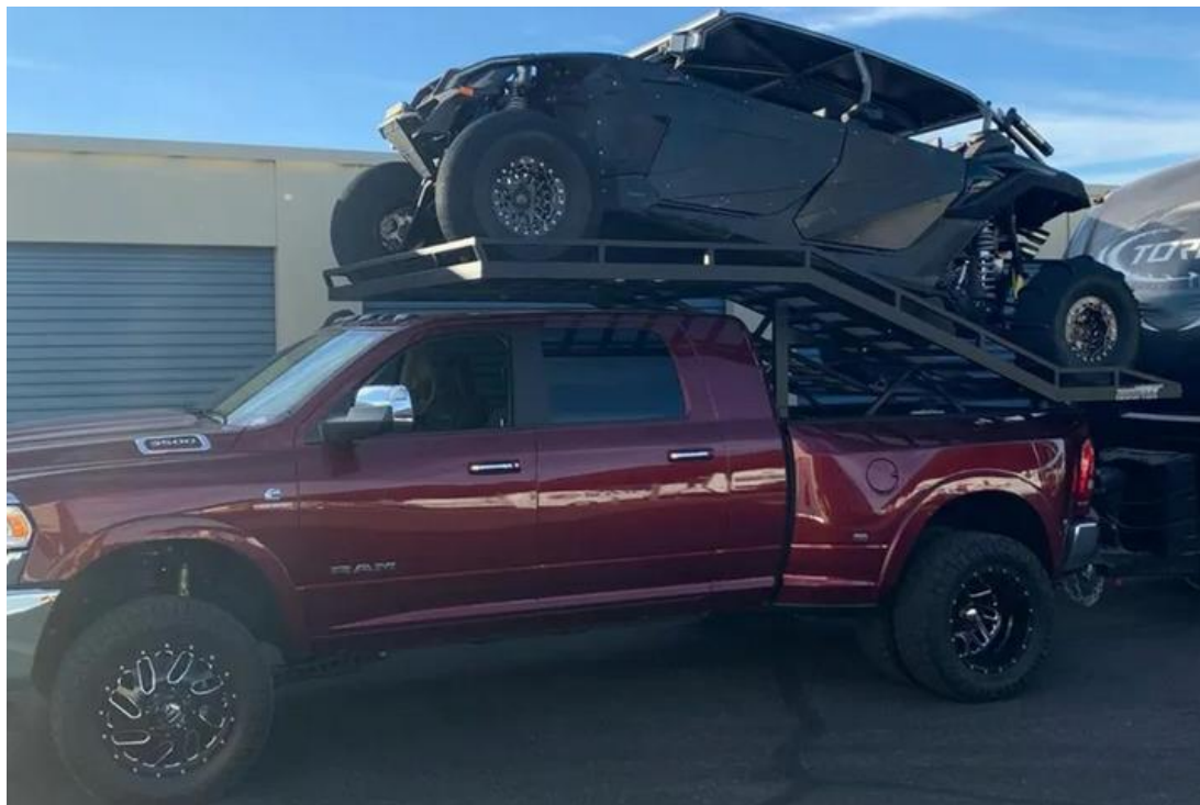
Dual Cab Max, Short Truck Bed, Dually, 4 Door UTV/Side by Side Truck Rack
